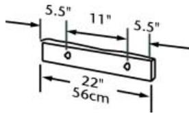
Drill two 1½" (28 - 30mm) dia. holes, 11" (28cm) apart and 5½" (14cm) in from each end and 1½" (38mm) down from top.
