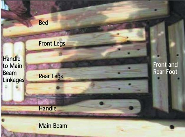
An Illustration of the Fuel Briquette Wood Parts
