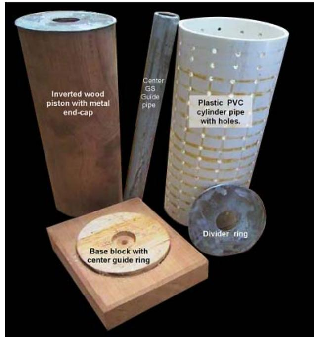
6. **Center guide ring:**  $\frac{1}{4}$  inch (6mm) thick. This ring is similar in dimensions to the above metal washers - 4 inches (10cm) diameter -with an inside hole diameter of  $1\frac{1}{8}$  inches (29 -30mm), however it is made of wood or plastic, not metal. This guide ring centers the cylinder and the guide pipe on the base plate.
