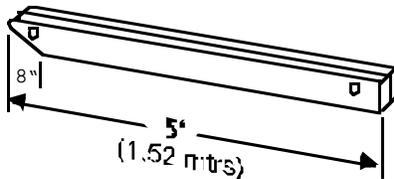
Left Side Top - 1" (25mm) radius on beam end.
