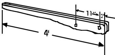
Drill two 1 1/8" (28 - 30mm) dia. holes, One on right is 2" (5cm) in from right end and 1 1/2" (38mm) down from top. Other is 13" (33cm) in from right end and 1 1/2" up from the bottom. Holes are 11" (28cm) apart.
